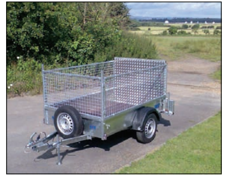
MEG7564TRM (Above) fitted with 145 R 13 Tyres, Loading Ramp, Weld Mesh Side Extension Kit and Rear Prop Stand Options
