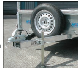
Optional Cast Coupling and Jockey Wheel shown on MEG7564WRM with 20.5 x 8 - 10 Tyres
