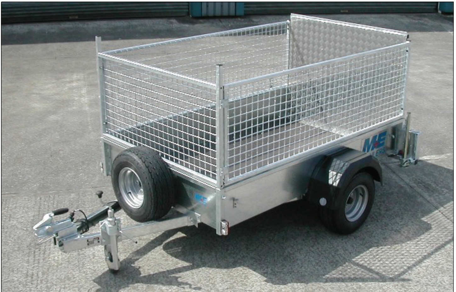
MEG7564WRM fitted with 20.5 x 8-10 Tyres, Loading Ramp and Weld Mesh Side Extension Kit, with Cast Coupling, Jockey Wheel and Rear Prop Stand Options.
