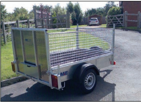
MEG7564TRM (Above) fitted with 145 R 13 Tyres, Loading Ramp, Weld Mesh Side Extension Kit and Rear Prop Stand Options
