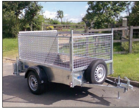
MEG7564TRM (Above) fitted with 145 R 13 Tyres, Loading Ramp, Weld Mesh Side Extension Kit and Rear Prop Stand Options
